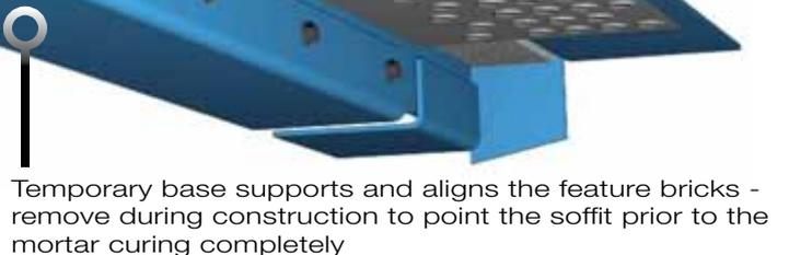
Temporary base supports and aligns the feature bricks -
